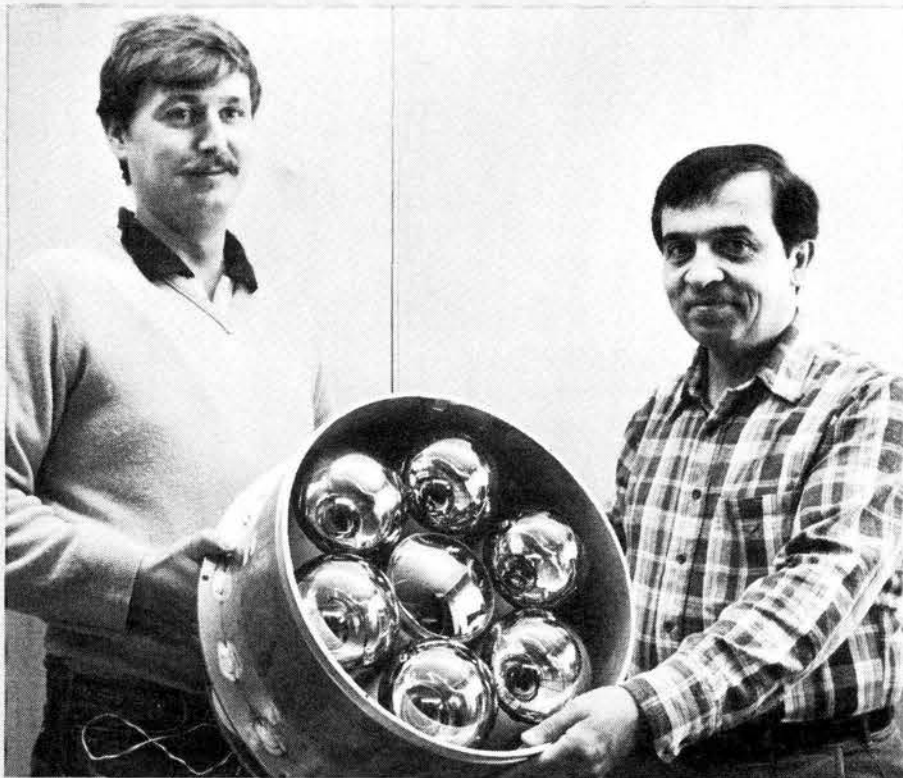
NOT A CHRISTMAS ORNAMENT but an array of photomultiplier tubes is what Jan Siemieniowski (left) and Tümay Tümer are getting ready to place into the solar collector. The device concentrates Cherenkov radiation to improve detectability of gamma ray showers from a faraway star.
